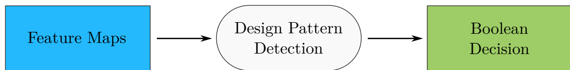
Figure 5.1.: The feature extraction process uses the feature maps and convolves over them. This results into a likelihood that the given map is of a certain pattern and ultimately to the boolean decision whether it is accepted or not.
